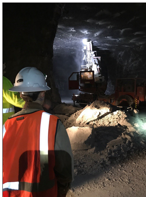
NMS student observing roof bolted in underground mine.
